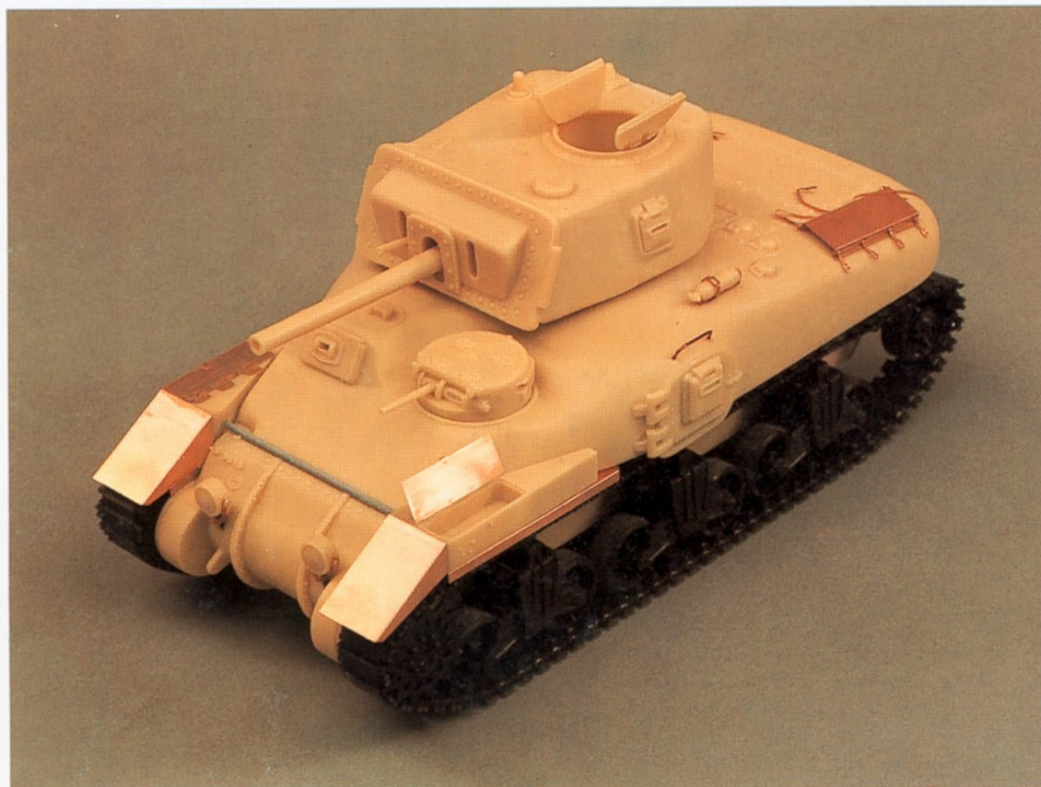
Fig.1 Completed model prior to airbrushing. The tracks are shown being test fitted.
